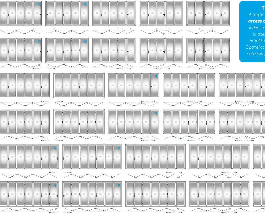
**Traffic Door!** A traffic door is an **every day access door**, that can be used independently without having to open all of the door set. Bi-fold doors fold in pairs, ie, a 3 panel configuration access door naturally falls to the left or right.
